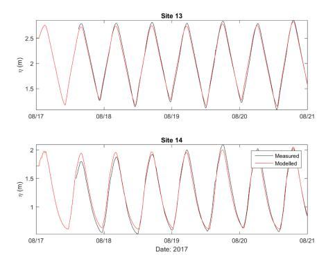
Figure A-7: Measured (black) and modelled (red) sea surface elevations for period 17 - 21 August 2017 for: Site 13 and Site 14.
