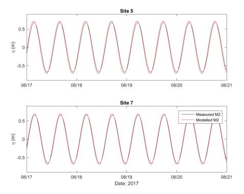
Figure A-2: Measured (black) and modelled (red)  $M_2$  tidal elevation predictions for the period 17 - 21 August 2017 for: Site 5 and Site 7.
