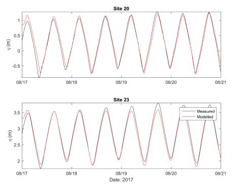
Figure A-9: Measured (black) and modelled (red) sea surface elevations for period 17 - 21 August 2017 for: Site 20 and Site 23.
