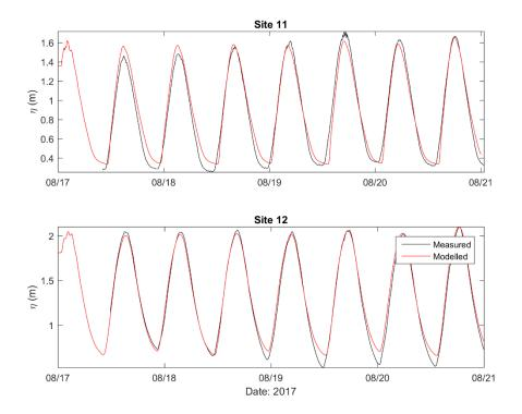
Figure A-6: Measured (black) and modelled (red) sea surface elevations for period 17 - 21 August 2017 for: Site 11 and Site 12.
