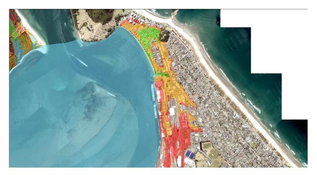
**Figure 8-4:** Modelled storm-tide inundation at Mount Maunganui. Blue marks inundation from 1% AEP storm-tide at 2020 MSL, green + 0.4 m SLR, orange +1.25 m SLR, red +1.6 m SLR.
