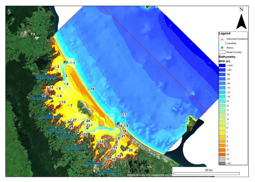
**Figure 3-1:** Tauranga Harbour inundation model bathymetry. The white triangles indicate the locations of available instrument data, the blue circles illustrate the most upstream river boundary locations incorporated into the model domain and the black line represents the model domain boundary. The bathymetry/digital elevation model overlays aerial photos and includes values of elevations from +15 m to depths < -200 m.
