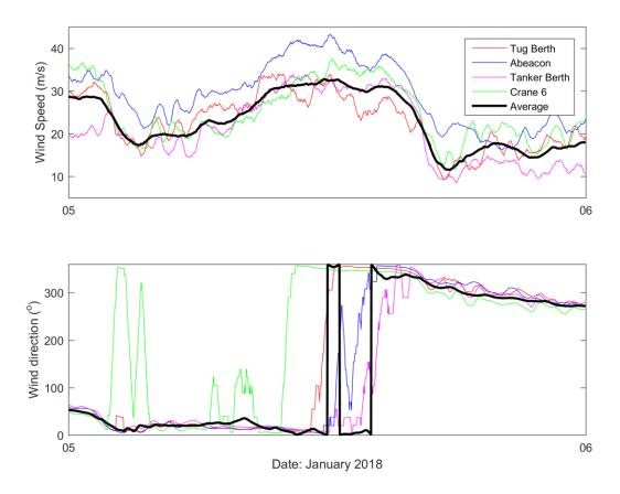
**Figure 4-2:** Wind speeds and directions recorded at Port of Tauranga weather stations on 5 January 2018. The bold line shows 1-hour running vector-average of the four sites, with peak wind speed of 32.7 m/s
