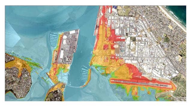
**Figure 8-3:** Modelled storm-tide inundation at Port of Tauranga. Blue marks inundation from 1% AEP storm-tide at 2020 MSL, green + 0.4 m SLR, orange +1.25 m SLR, red +1.6 m SLR.
