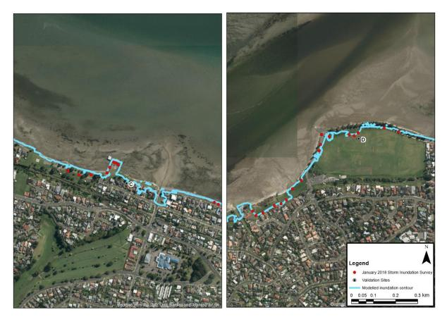
**Figure 4-6:** Model validation for the horizontal extent of inundation during 5 January 2018 storm-tide, at sites C **(Otumoetai) and D (Tilby Point).** The light blue line represents the modelled predict inundation extent and the red dots are measured inundation heights and extents.
