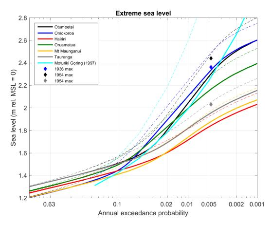
**Figure 8-4:** Extreme sea levels in Tauranga Harbour. Sea levels require the addition of MSL to make them relative to MVD–53. Dashed lines represent upper 95% confidence intervals. Extreme sea levels were calculated using the SSJPM method, except at Moturiki where the Goring et al. (1997) RJPM results are used. Historic maxima are plotted using Gringorten (1963) plotting position for the annual maximum in a 120-year sequence.
