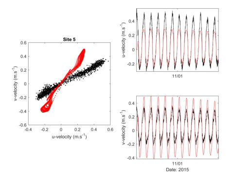
Figure B-7: Measured (red) and modelled (black) depth-averaged u and v components of velocity at Site 5 for the 10 October - 4 November 2015.
