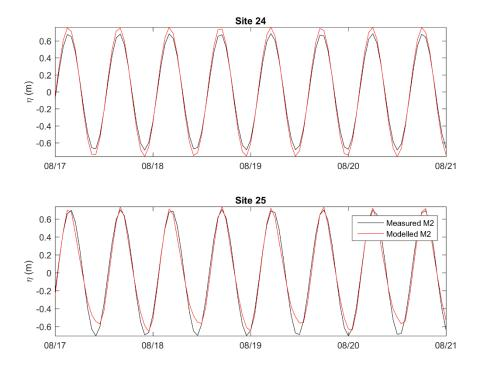
Figure A-3: Measured (black) and modelled (red) M<sub>2</sub> tidal elevation predictions for the period 17 - 21 August 2017 for: Site 24 and Site 25.
