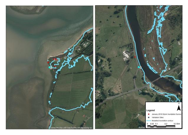
**Figure 4-9:** Model validation for the horizontal extent of inundation during 5 January 2018 storm-tide, at sites I (Waikareao Estuary) and J (Wairoa River). The light blue line represents the modelled predict inundation extent and the red dots are measured inundation heights and extents.
