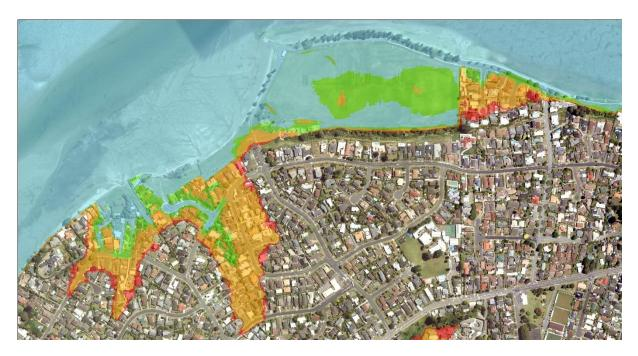
**Figure 8-2:** Modelled storm-tide inundation at Otumoetai. Blue marks inundation from 1% AEP storm-tide at 2020 MSL, green + 0.4 m SLR, orange +1.25 m SLR, red +1.6 m SLR.
