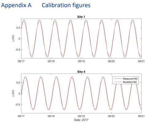
Figure A-1: Measured (black) and modelled (red) M<sub>2</sub> tidal elevation predictions for the period 17 - 21 August 2017 for: Site 1 and Site 4.
