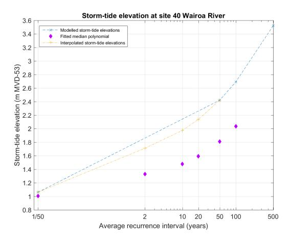
**Figure 12-3: Demonstration of interpolation method.** The blue crosses mark the model results from Reeve et al. (2018). The yellow crosses mark the interpolated elevations at 39, 10 and 5% AEP, obtained by scaling the median fitted polynomial to match the model results at ARI of 1/50 and 50 years. Purple diamonds mark the median extreme sea-level polynomial fit.
