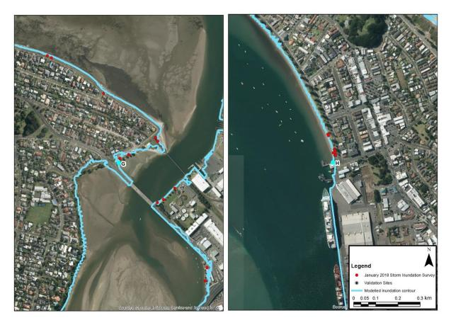
**Figure 4-8:** Model validation for the horizontal extent of inundation during 5 January 2018 storm-tide, at sites G (North Waikareao Estuary) and H (Pilot Bay). The light blue line represents the modelled predict inundation extent and the red dots are measured inundation heights and extents.
