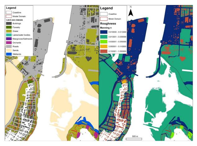
Figure 2-2: Spatially varying land use classification created from the support vector machine analysis (Left-hand-side), and illustration of the conversion from land use to Manning's n (Right-hand-side).
