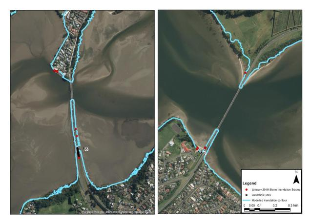
**Figure 4-5:** Model validation for the horizontal extent of inundation during 5 January 2018 storm-tide, at sites A (Hairini Bridge) and B (Maungatapu). The light blue line represents the modelled predict inundation extent and the red dots are measured inundation heights and extents.
