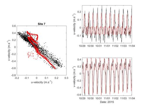
Figure B-9: Measured (red) and modelled (black) depth-averaged u and v components of velocity at Site 7 for the 10 October - 4 November 2015.
