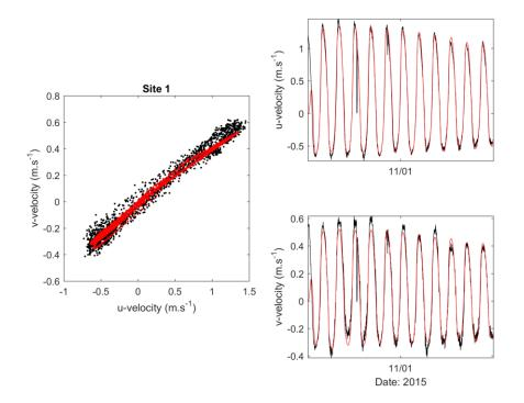
Figure B-3: Measured (red) and modelled (black) depth-averaged u and v components of velocity at Site 1 for the 10 October - 4 November 2015.
