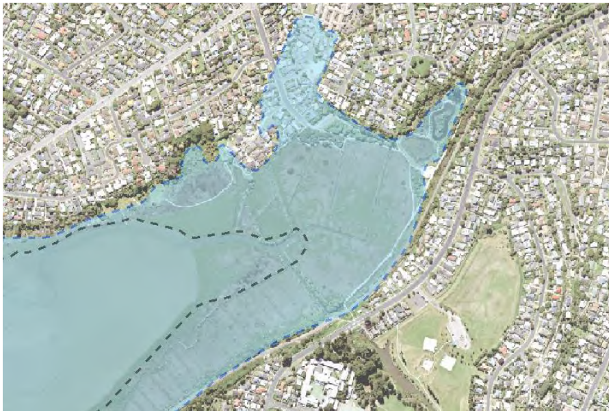
Figure 5-8 Example of how low-lying estuarine shorelines are likely to be translated landward with inundation from future SLR scenarios (black dashed line represents the current MHWS, blue shading represents future MHWS with 1.6 m SLR).
