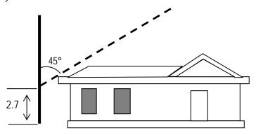
Figure 1: Daylighting Calculation
