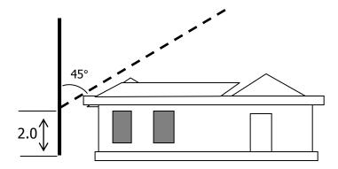
Figure 1: Daylighting Calculation
