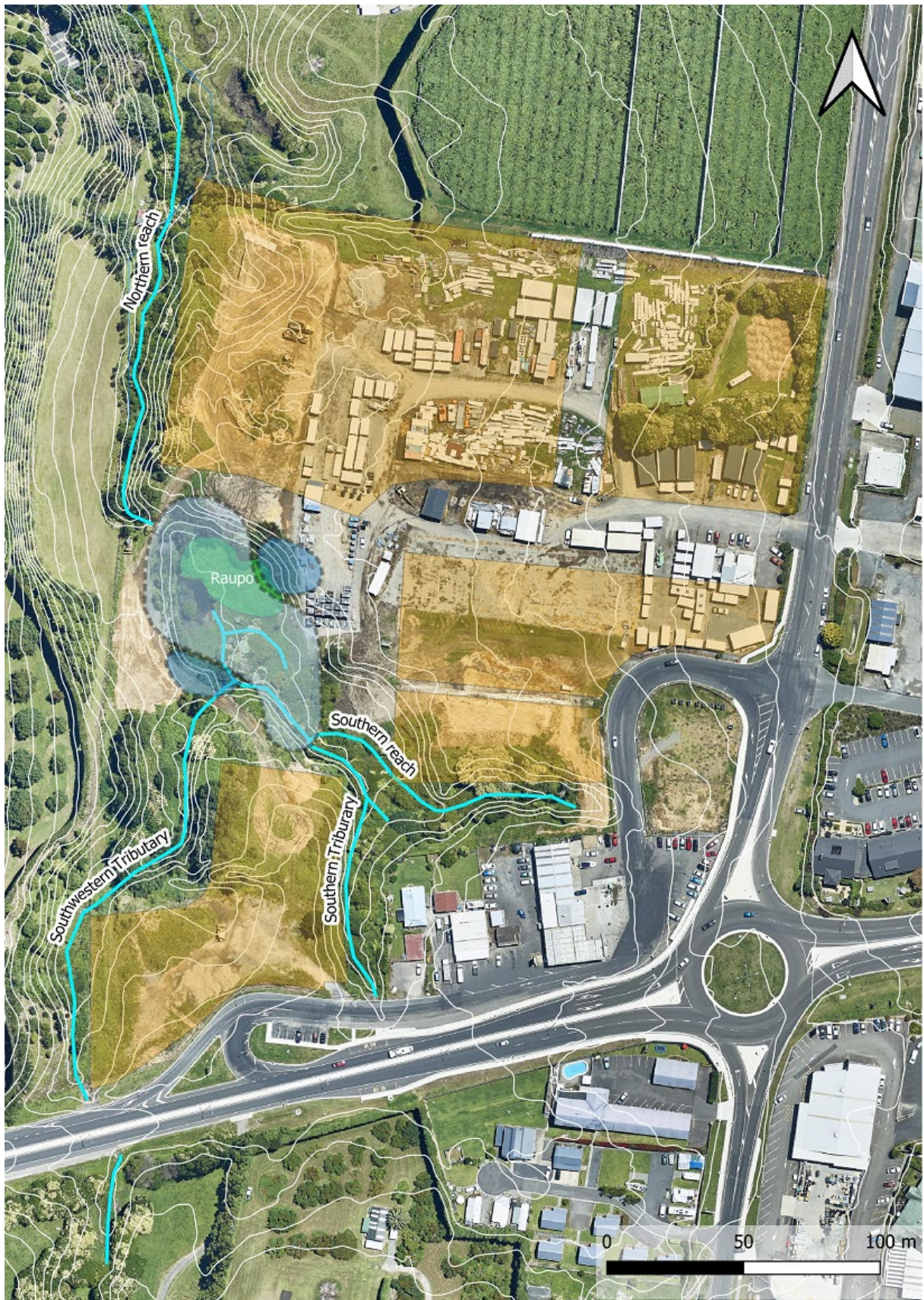
Figure 1: Te Puna Springs Estate location of stream network, the raupo wetland, proposed commercial development layout, ponds and treatment wetlands.
