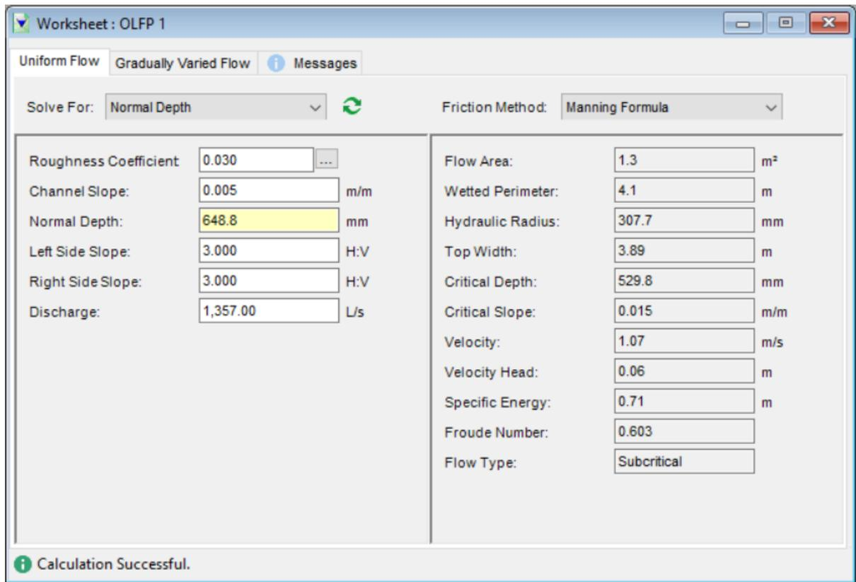
Figure 7: Flowmaster results of required flow depth for OLFP 1 in the secondary storm event, assuming a 0.5% channel grade triangular channel (no bottom width)
