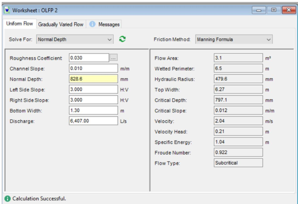
Figure 8: Flowmaster results of required flow depth for OLFP 2 in the secondary storm event, assuming a 1.3m base width and 1% channel slope in a trapezoidal channel
