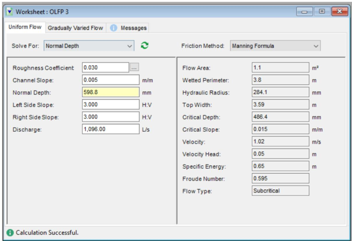
Figure 9: Flowmaster results of required flow depth for OLFP 3 in the secondary storm event, assuming a 0.5% channel grade triangular channel (no bottom width)
