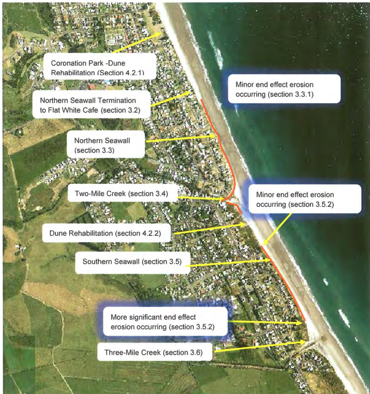
Figure 2 – Seawall and Dune Rehabilitation Areas including report section references
