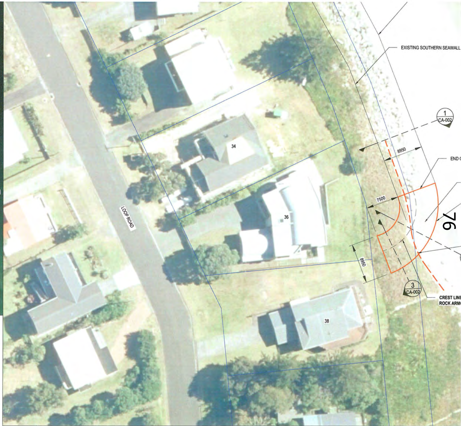
B SOUTHERN SEAWALL TERMINATION CA-001 SCALE 1:500 (A3)
