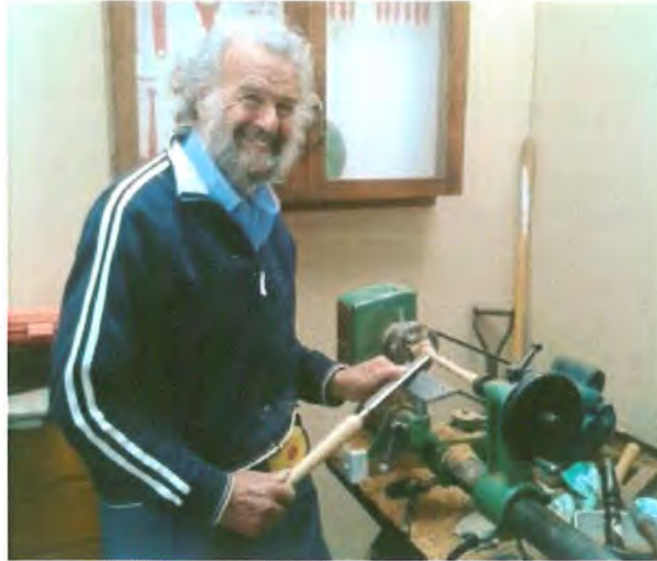
George turning a cipin (drum stick). Note: Safety equipment removed for photo
