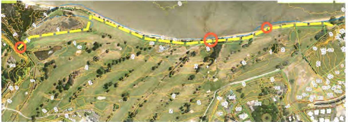
Approximate location of bund and walkway. Red rings denote storm water outlets.
