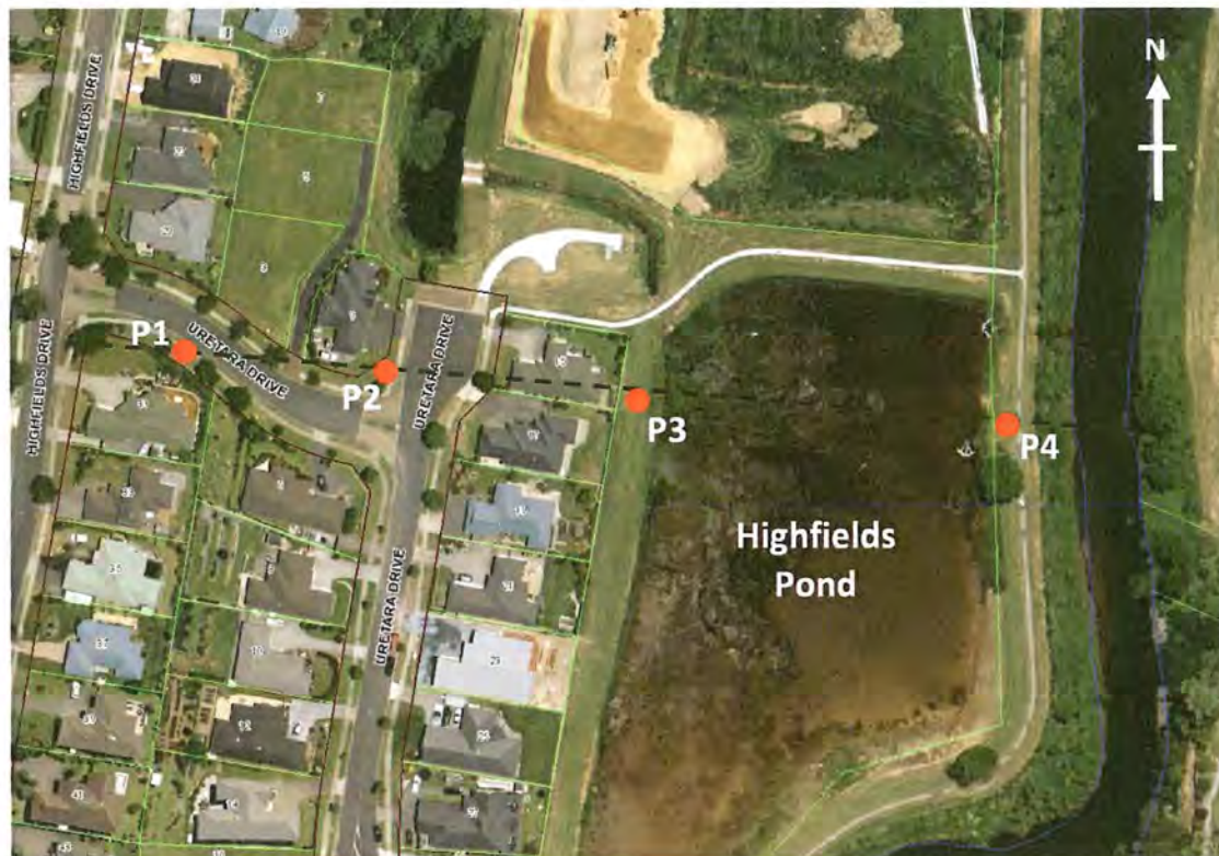
Figure 3.1: Groundwater monitoring locations
