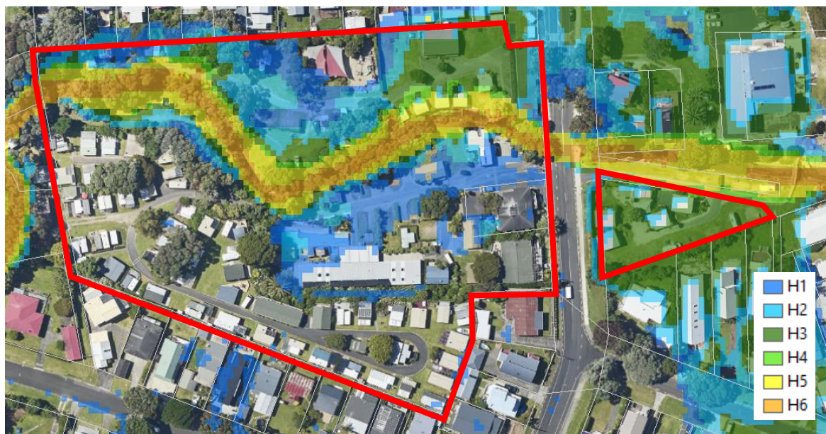
Figure 3.1: Top 10 Campground flood hazard categorisation for a 1% AEP present day storm event (property boundary in red)
