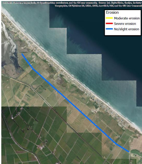
Figure 3. Map showing stream bank erosion of the unnamed canal in the Pukehina Catchment.
