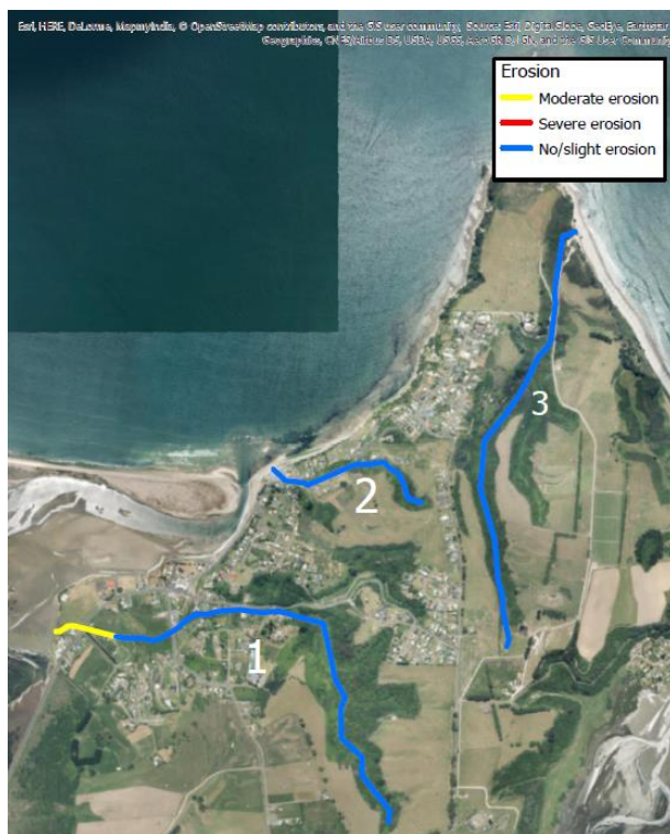
Figure 2 - Map showing stream bank erosion of streams surveyed in the Maketu Catchment. 1 - Little Waihi Road Stream. 2 - Town Point Road Stream. 3 - Nedwicks Beach Stream.
