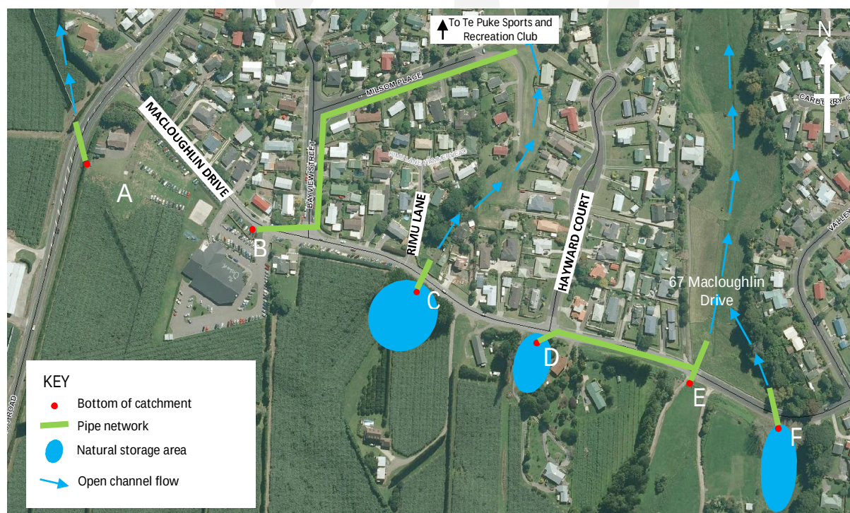
Figure 5: Existing stormwater infrastructure
