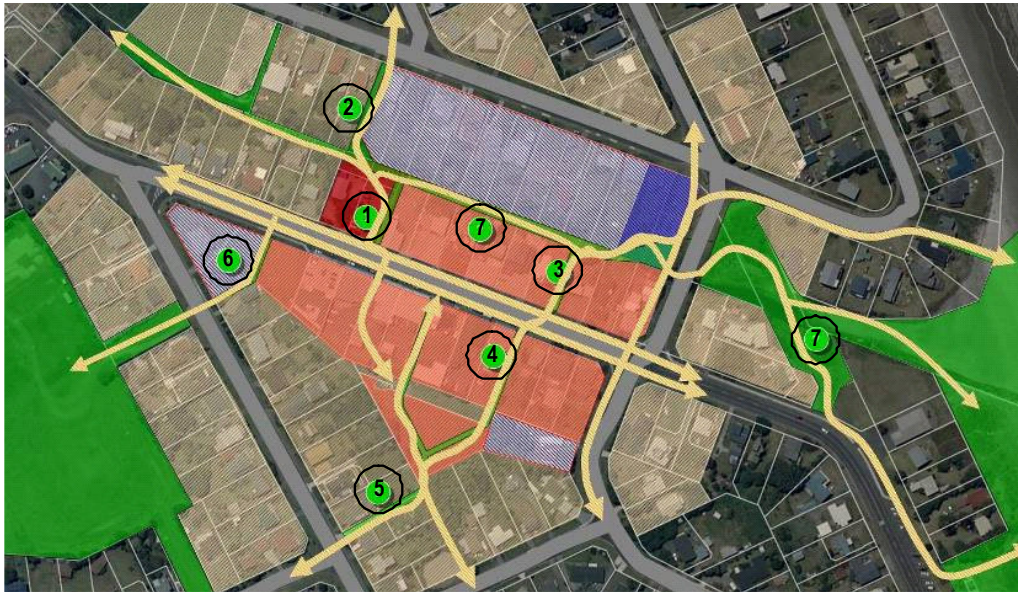
4.9 The proposed footpath network (above) linking the town centre and the two focal points (indicated in red and blue) through the open space network to its population catchment. The footpath routes potentially have different methods to secure them like 'overlay' zones or acquisition.
