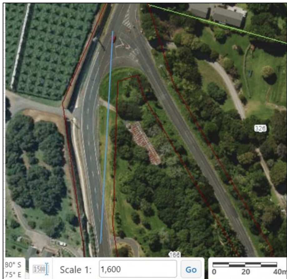
Figure 20: Sight line to intersection that might be available if there is no traffic in the southbound lane and if there are no obstructions in the opposing berm (approximately 130m). Note that this is not how standard sight distance is measured.
