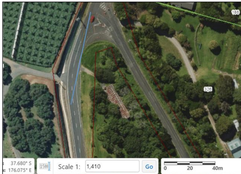
Figure 19: Sight line to intersection that might be available if there is no traffic in the southbound lane (approximately 77m). Note that this is not how standard sight distance is measured.
