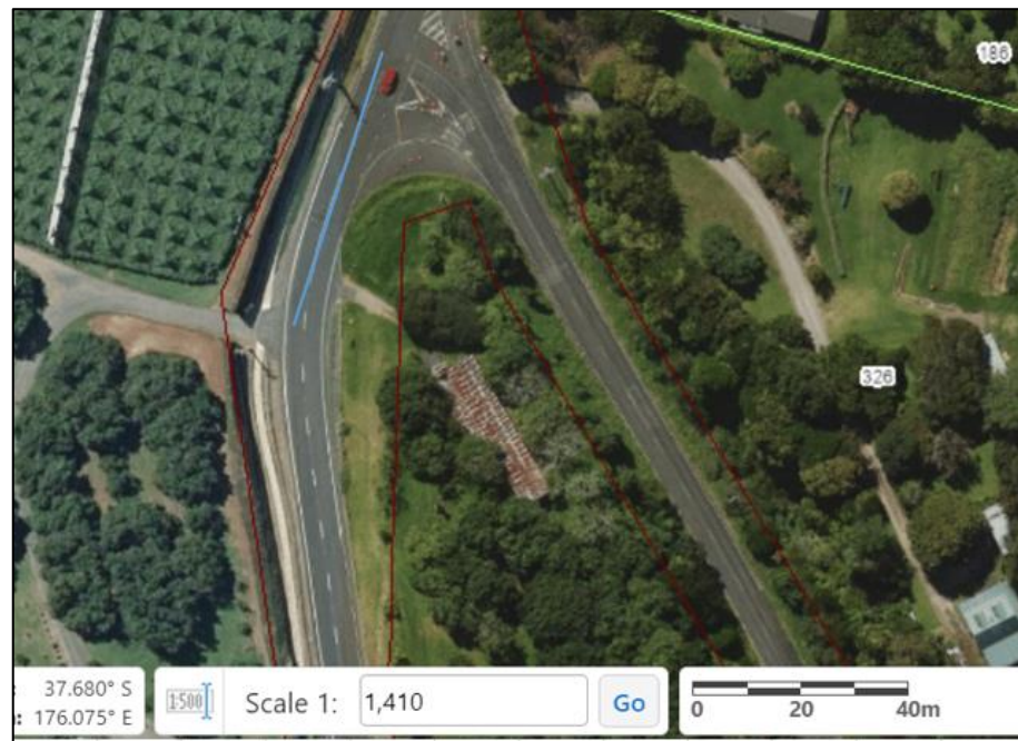
Figure 18: Sight line to intersection is shown by the blue line (approximately 60m long).
