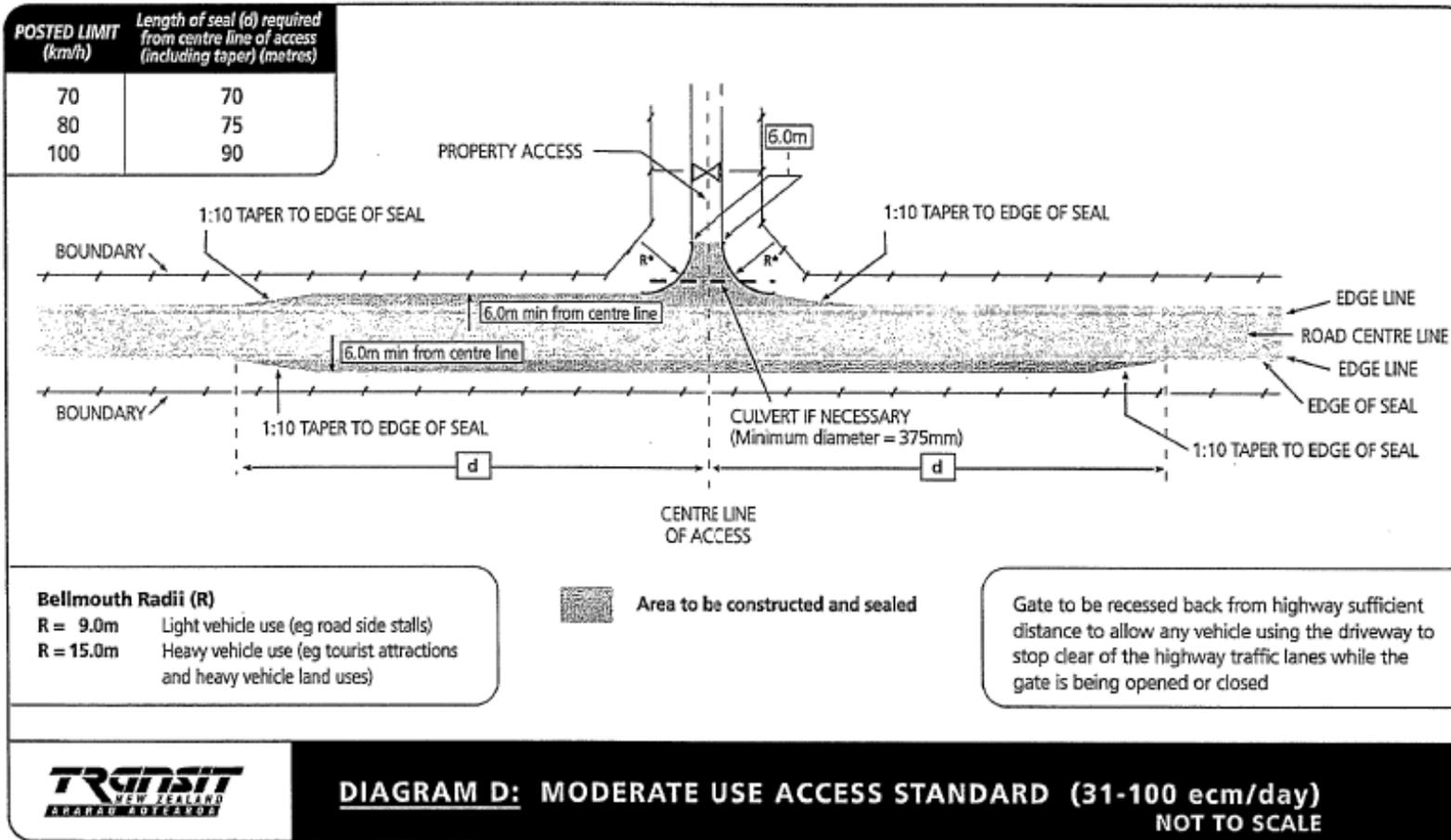
Figure 1: Access layout diagram for 31-100 ecm/day from the 1999 PPM
