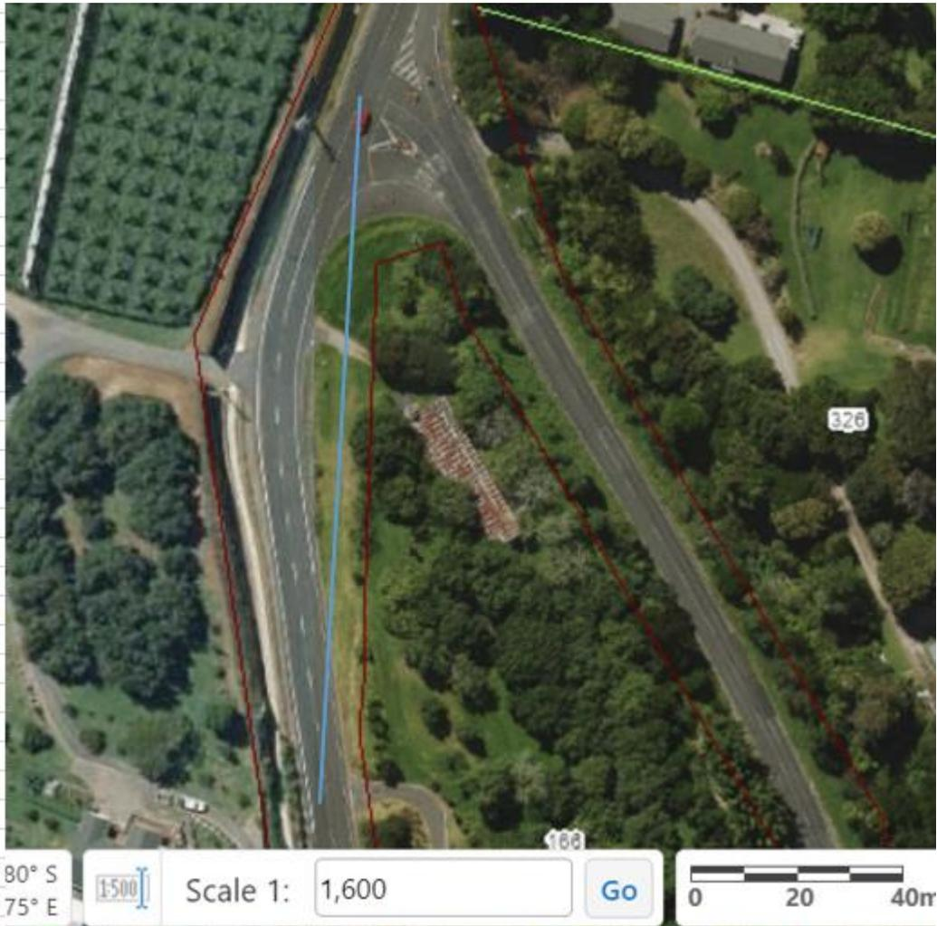
Figure 22: Sight line to intersection that might be available if there is no traffic in the southbound lane and if there are no obstructions in the opposing berm (approximately 130m). Note that this is not how standard sight distance is measured.
