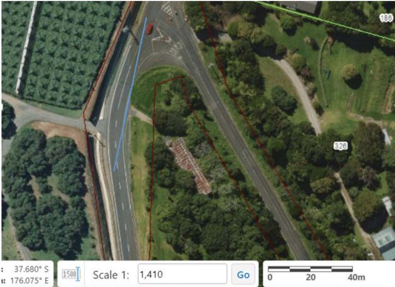
*Figure 21: Sight line to intersection that might be available if there is no traffic in the southbound lane (approximately 77m). Note that this is note how standard sight distance is measured.*
