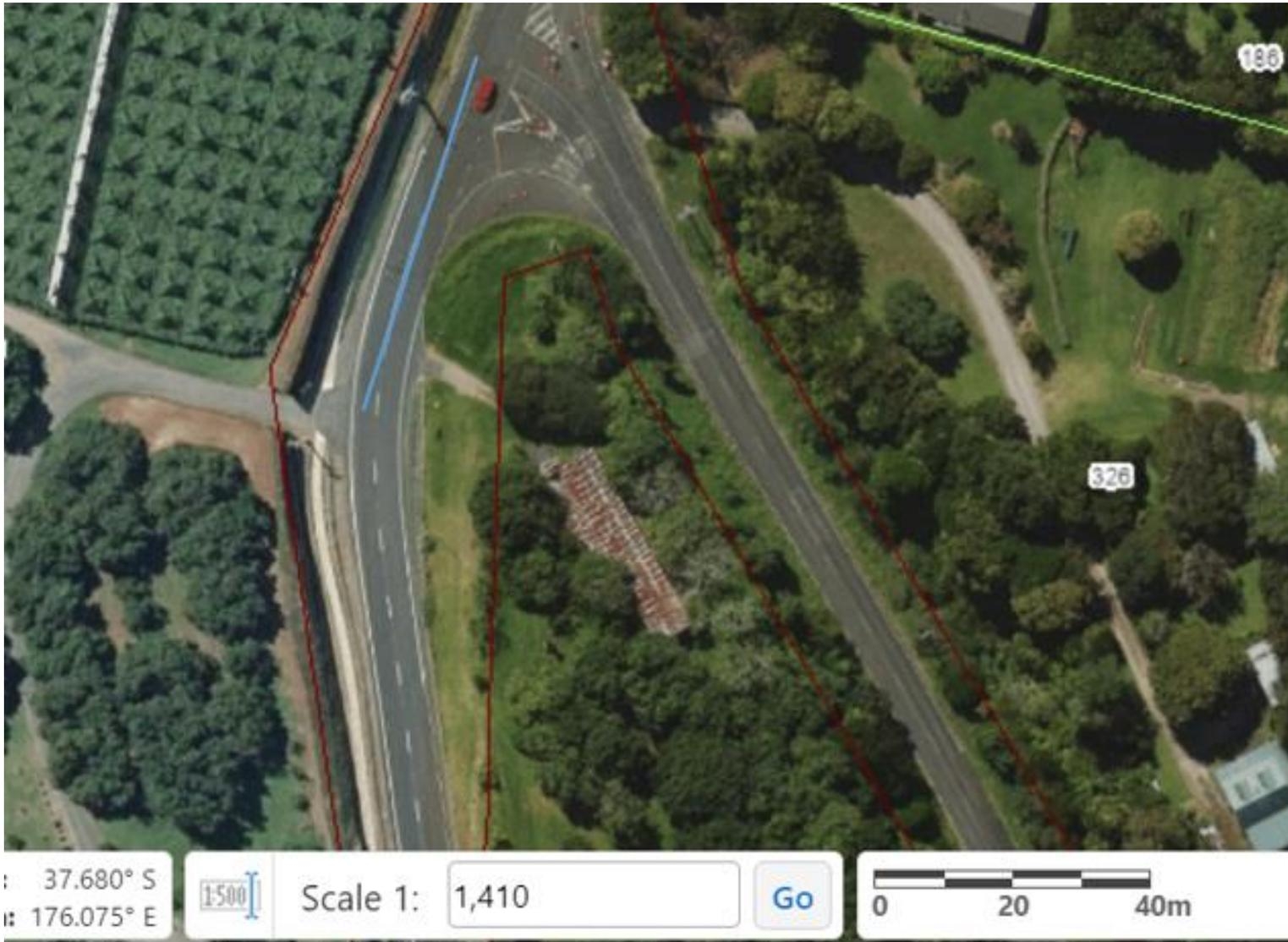
Figure 20: Sight line to intersection is shown by the blue line (approximately 60m long).
