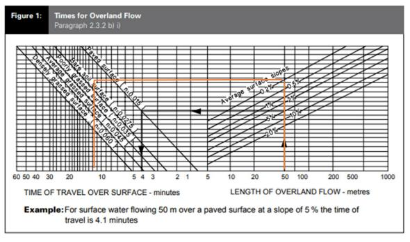
The overall time of concentration is therefore considered to be in the order of 17 minutes, which is at least equivalent for the undeveloped original site.
