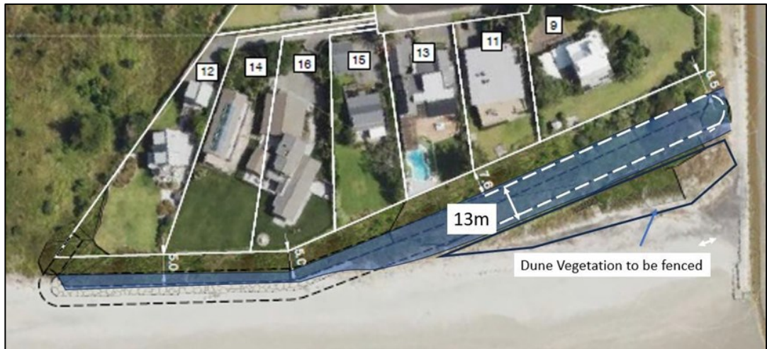
Figure 14: Indicative location of vegetation removal (blue), proposed structure (black dashed line) and northern dune vegetation to be protected.
