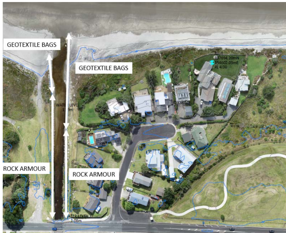
Figure 3.4a: Armouring to 3 Mile Creek
