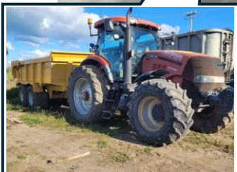
PNEUMATIC WHEELED TRACTOR AND TRAILER DELIVER ROCKS TO THE BEACH FRONT WORK AREA
