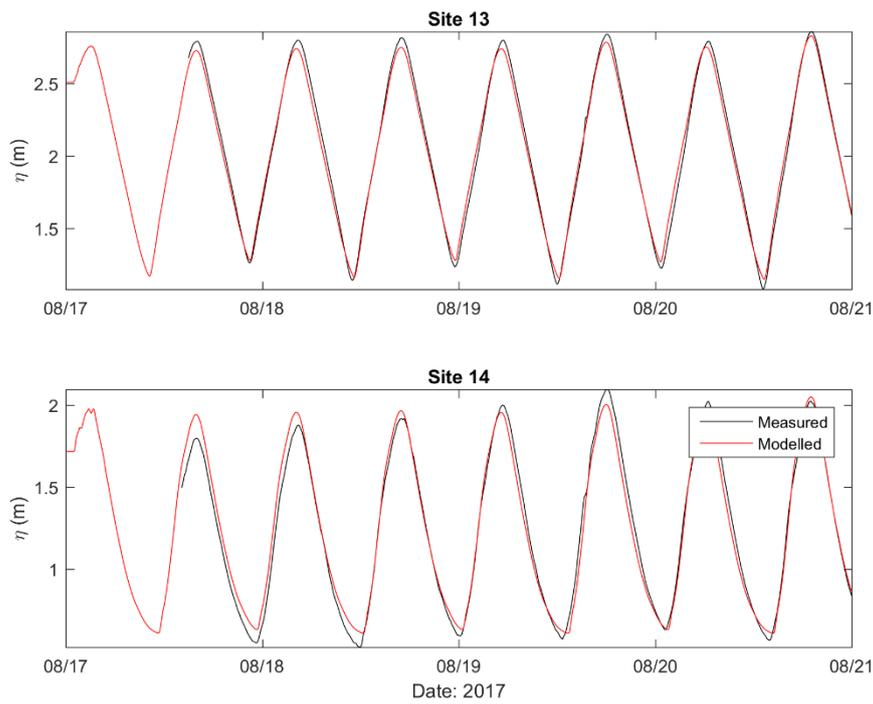
**Figure A-7: Measured (black) and modelled (red) sea surface elevations for period 17 - 21 August 2017 for: Site 13 and Site 14.**
