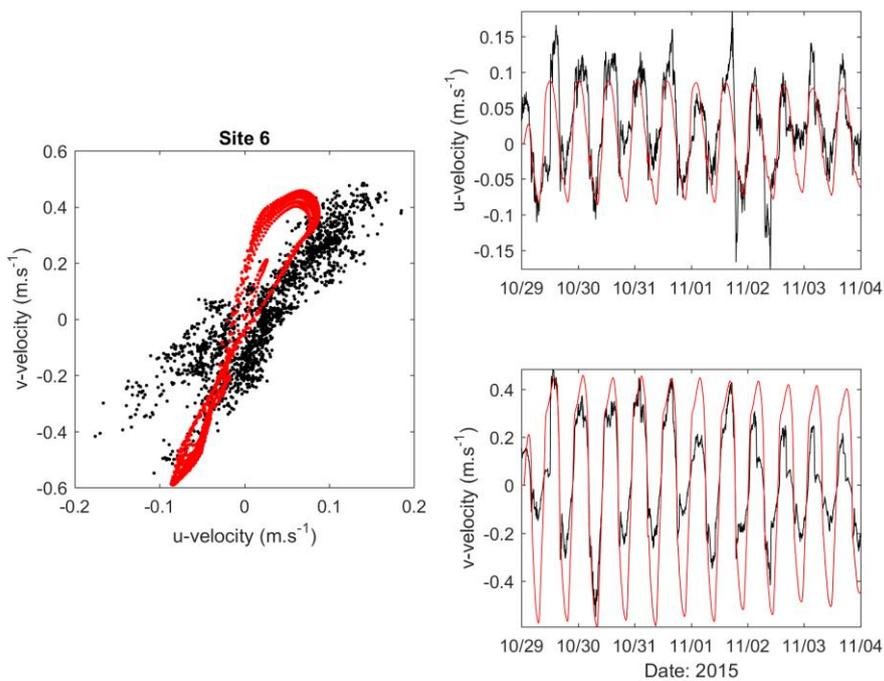
**Figure B-8: Measured (red) and modelled (black) depth-averaged u and v components of velocity at Site 6 for the 10 October - 4 November 2015.**
