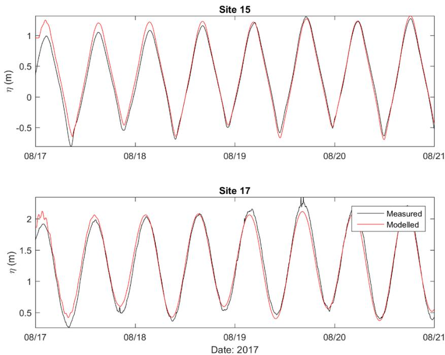
**Figure A-8: Measured (black) and modelled (red) sea surface elevations for period 17 - 21 August 2017 for: Site 15 and Site 17.**
