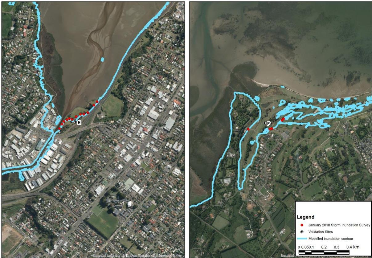
**Figure 4-7: Model validation for the horizontal extent of inundation during 5 January 2018 storm-tide, at sites E (South Waikareao Estuary) and F (Omokoroa Golf Course). The light blue line represents the modelled predict inundation extent and the red dots are measured inundation heights and extents.**
