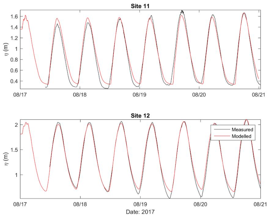
**Figure A-6: Measured (black) and modelled (red) sea surface elevations for period 17 - 21 August 2017 for: Site 11 and Site 12.**
