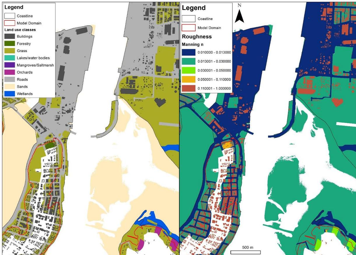
**Figure 2-2: Spatially varying land use classification created from the support vector machine analysis (Left-hand-side), and illustration of the conversion from land use to Manning's n (Right-hand-side).**
