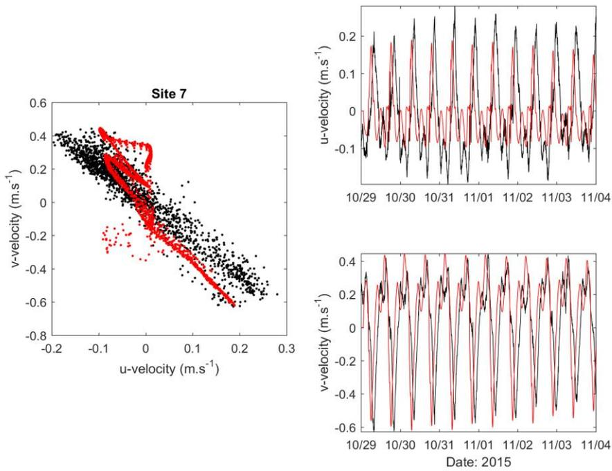
**Figure B-9: Measured (red) and modelled (black) depth-averaged u and v components of velocity at Site 7 for the 10 October - 4 November 2015.**
