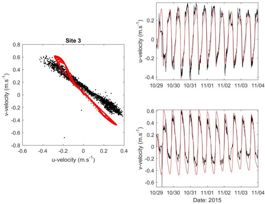
**Figure B-5: Measured (red) and modelled (black) depth-averaged u and v components of velocity at Site 3 for the 10 October - 4 November 2015.**
