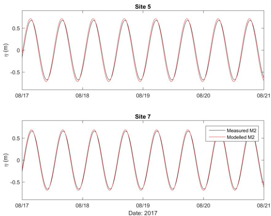
**Figure A-2: Measured (black) and modelled (red) M<sub>2</sub> tidal elevation predictions for the period 17 - 21 August 2017 for: Site 5 and Site 7.**
