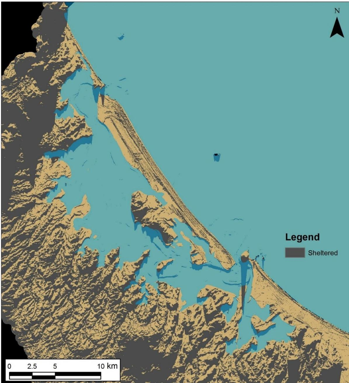
**Figure 4-3: Example of the North wind shadowing.** Using the Viewshed 2 ARC GIS tool locations sheltered from north, north-northeast and north-easterly (onshore) wind directions were identified.
