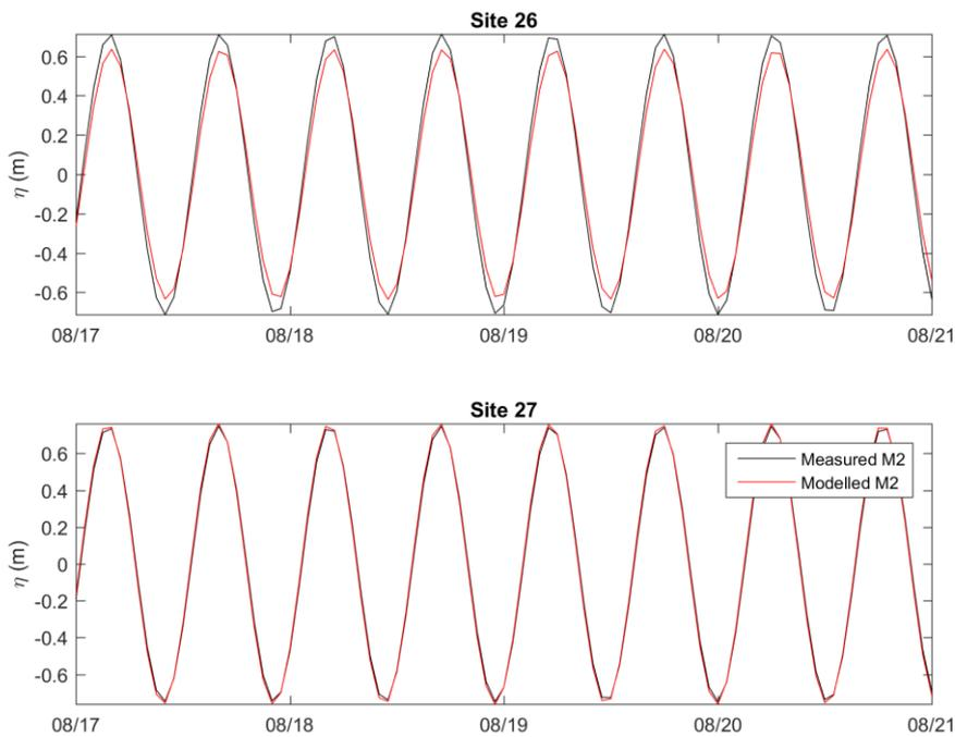
**Figure A-4: Measured (black) and modelled (red) M<sub>2</sub> tidal elevation predictions for the period 17 - 21 August 2017 for: Site 26 and Site 27.**
