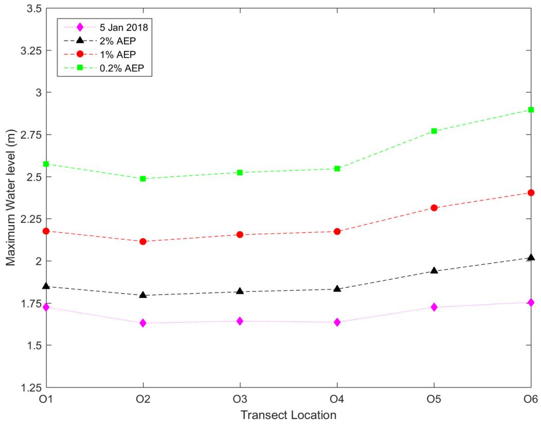
**Figure 5-8: Maximum water elevations extracted from transect "O".** Transect O runs from east (Sulphur Point) to west (Omokoroa), Figure 5-4.
