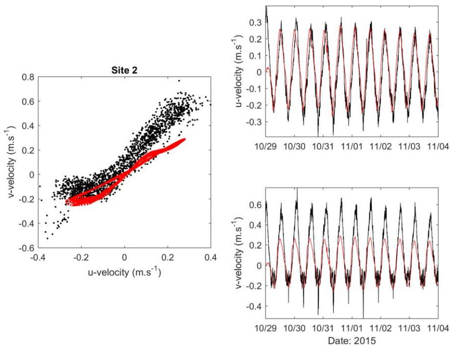
**Figure B-4: Measured (red) and modelled (black) depth-averaged u and v components of velocity at Site 2 for the 10 October - 4 November 2015.**
