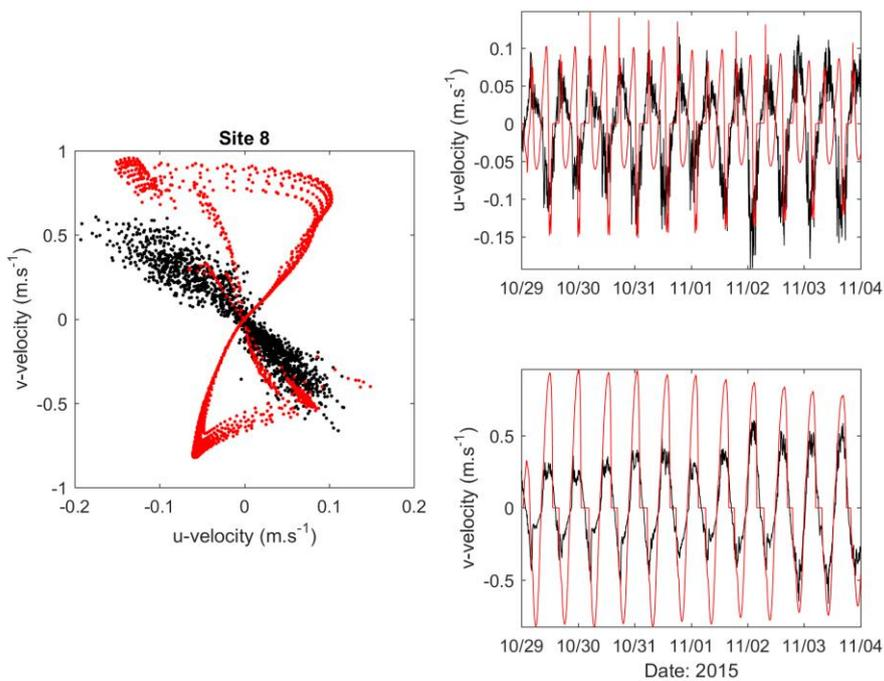
**Figure B-10: Measured (red) and modelled (black) depth-averaged u and v components of velocity at Site 8 for the 10 October - 4 November 2015.**
