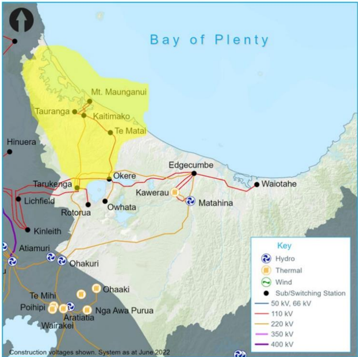
National Grid Assets in the Western Bay of Plenty (highlighted yellow)
