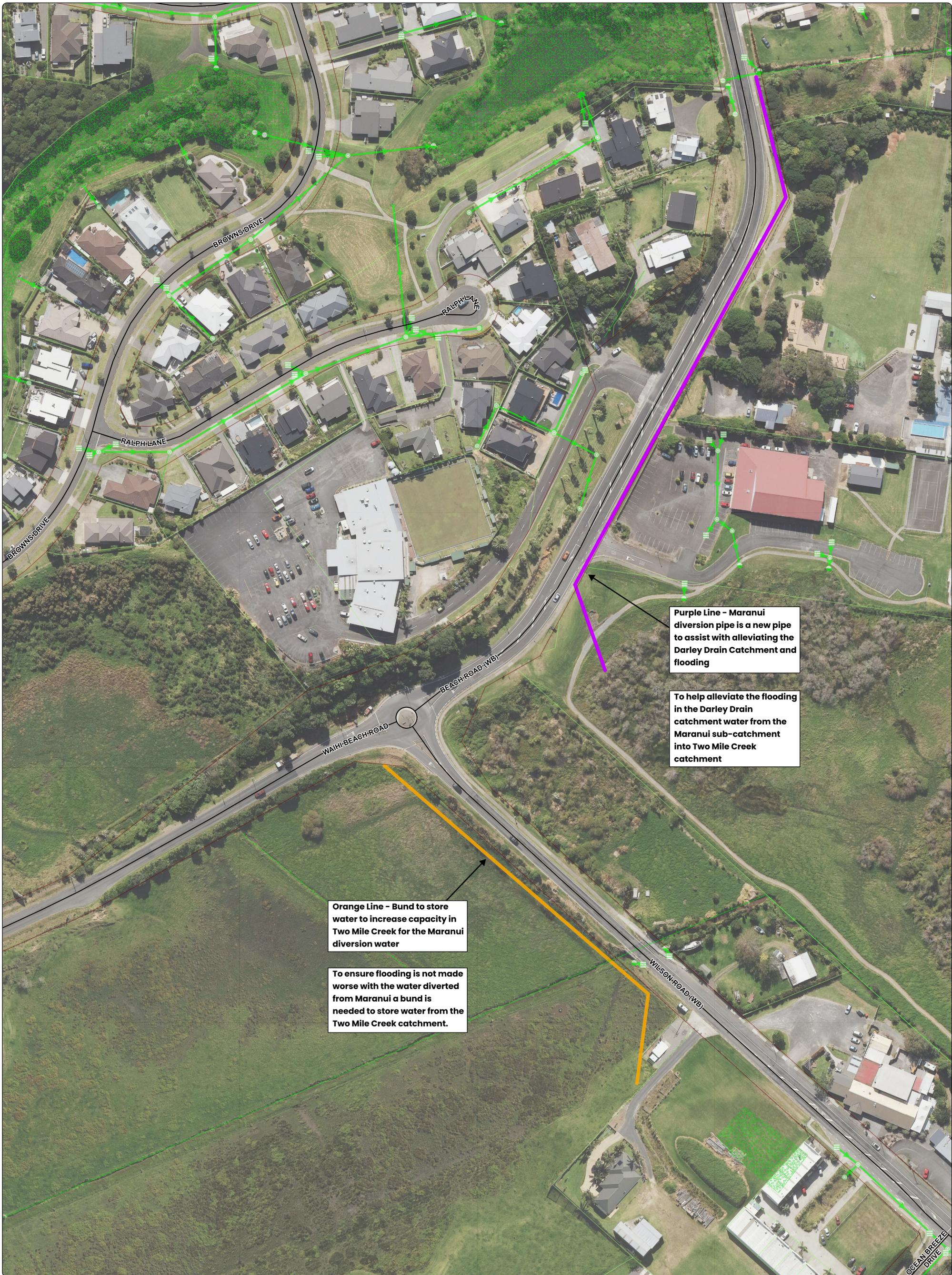
**Purple Line - Maranui diversion pipe is a new pipe to assist with alleviating the Darley Drain Catchment and flooding**
